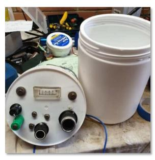
Once connected, I place the transmitter in "CW" and tune the GTU for maximum deflection. I do not worry about what the graduations are on my meter.
